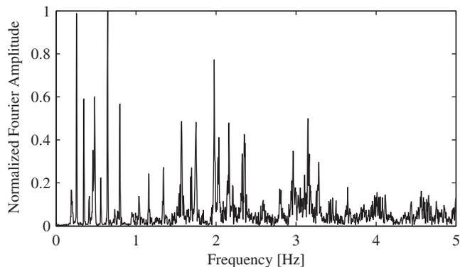
**Fig. 3.** Fourier amplitude spectrum of vertical acceleration response at Station 3SW measured during the ambient vibration test
