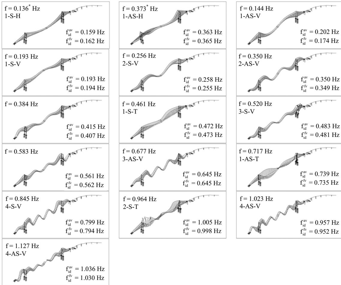
**Fig. 10.** Vibration mode shapes of the AZMB computed from the bridge FE model in ADINA (\*=horizontal vibration modes and  $f_{id}^{av}, f_{id}^{fv}$  = natural frequency identified based on ambient vibration and forced vibration data, respectively, averaged over the three system identification methods)
