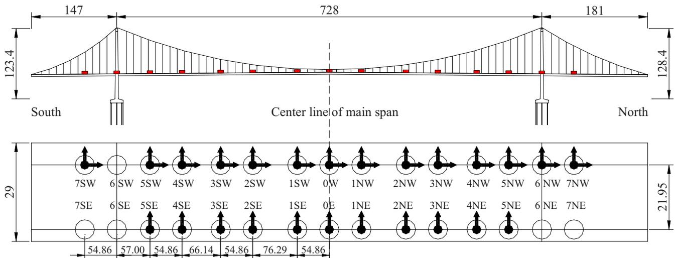
Fig. 1. Overall dimensions of the AZMB and instrumentation (accelerometers) layout (m)
