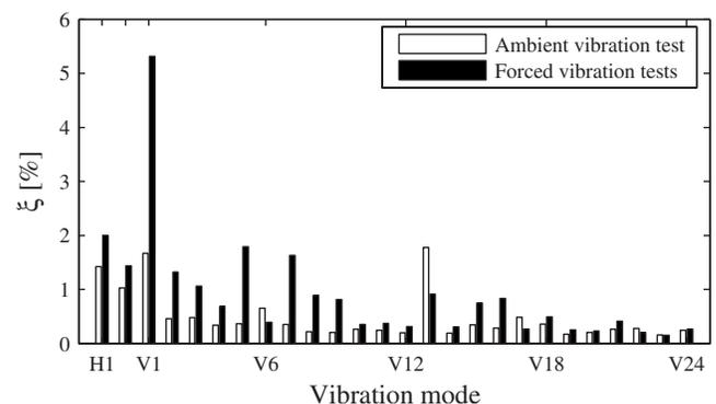
**Fig. 8.** Comparison of damping ratios identified using ambient vibration and forced vibration test data (see Fig. 6 or 7 for abbreviation of vibration modes)
